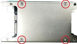
5. Install the bracket with the storage device back into the computer by refastening the 4 screws. Connect the SATA cable and power cable to the connectors on the computer.
