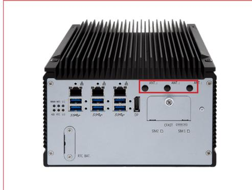
Arrange the flat side of the SMA connector to meet the flat side of the antenna hole.
