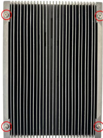
2. Carefully lift the top cover and remove the top cover from the computer. The inside of the computer is revealed.
