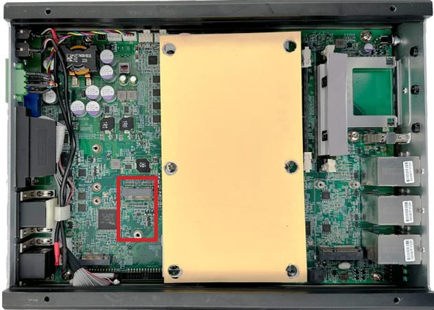
3. Prepare the Wi-Fi module kit. The module is a **M.2 E-Key** socket form factor, with two MHF connectors, one is “MAIN”, and the other is “AUX”.
