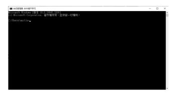
Step 3. Execute the application program by command Example. Command line  $\rightarrow$  FitCANBus.exe COM5 1000 12345678 29 0 0 0 0 0 FitCANBus.exe  $\rightarrow$  Execute the application program file name <COM Port Number>  $\rightarrow$  It depends on the COM PORT of the computer, the examples are com5 & com6. Example:
