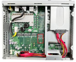
3. Prepare the Wi-Fi module kit. The module is a **M.2 E-Key** socket form factor, with two MHF connectors, one is "MAIN", and the other is "AUX".
