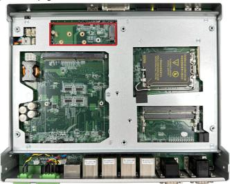
2. Insert the M.2 module into the socket by aligning the notch on the module with the small slot on the M.2 socket.
