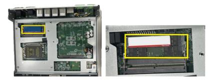
3. Install the NVMe SSD & SO-DIMM, which are close to the top case, then add the thermal pad and remove the thermal pad protection films.
