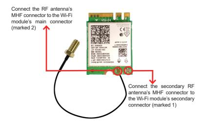
6. Plug the Wi-Fi module to the socket's connector by a slanted angle. Fully plug the module, and note the notch on the wireless module should meet the break of the connector.
