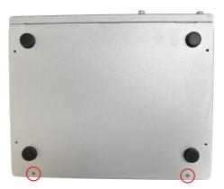
2. Carefully lift the bottom cover and then completely part the side cover from the computer.
