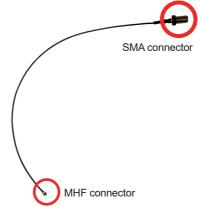
5. Connect the RF antenna's MHF connector to the Wi-Fi module's main connector marked 0. If you are going to connect a secondary antenna, connect it to the connector marked 1.
