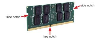
The computer has two 262-pin DDR5 SO-DIMM sockets that each socket support up to 64 GB maximum system memory. To install a memory module:
