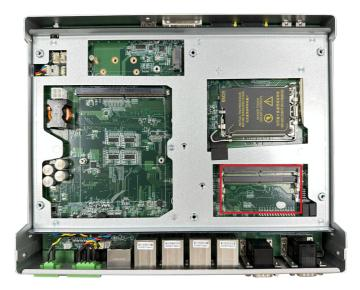
3. Align the notch on the memory module with the key in the module socket.
