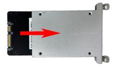
3. Fix the storage device in place by fastening the four screws of the bracket.
