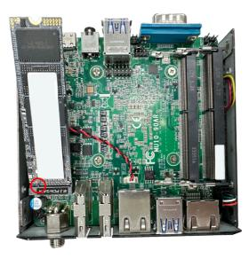
2. Press the module down and fix the module in place using one screw.
