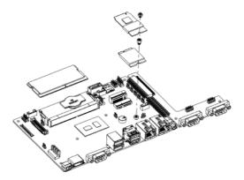
After installing M.2 device, please place the thermal pad on the M.2 module. Align thermal pad with the heat-generating area of the component and ensure that it covers the entire surface area that requires thermal contact. Once it is in position, apply gentle pressure to the component to ensure good contact and compression between the pad and the surface.
