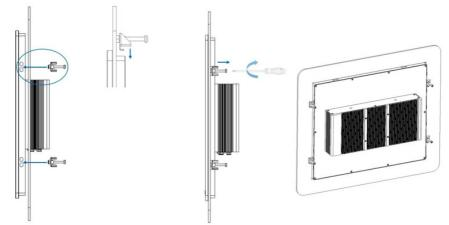
Attach the VESA bracket to the product's 75 x 75mm VESA hole by four screws.
